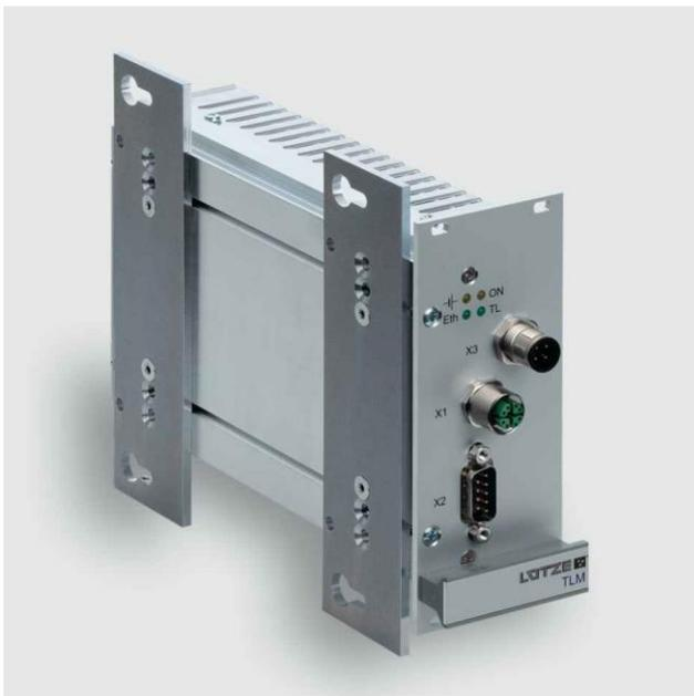
The device uses the existing NF cabling for data transmission. A tap-proof data transfer is guaranteed by a 128-bit AES encryption. The bandwidth of the transmission line is constantly determined via a DSP, which ensures an optimal data throughput.
